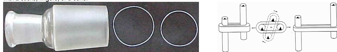
Picture left: Sealing ring diameter, decrease after warming. Picture right: Increasing the ring diameter by stretching.
